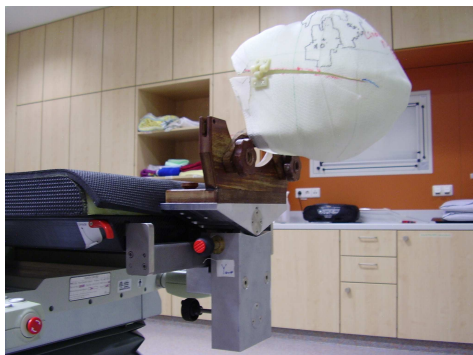
Figure 2: The adjustable mask-mount system. One can see the black knobs to adjust the angles.
